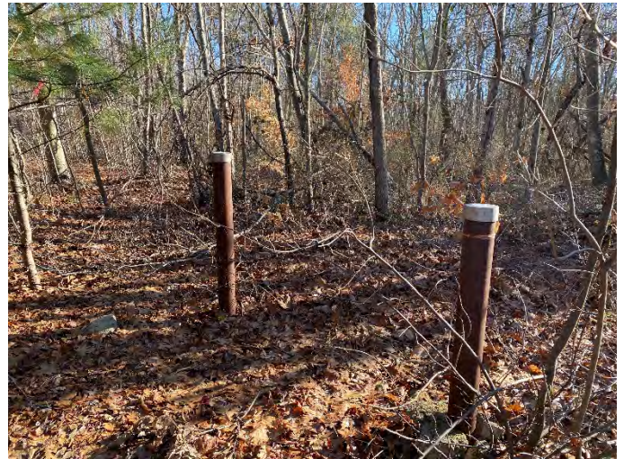
Photograph #26 Groundwater monitoring wells MW-5S and 5D in good condition and equipped with locks.
