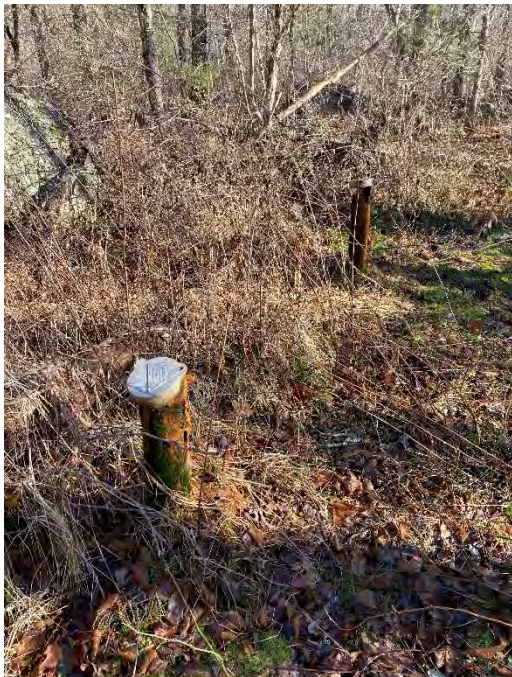
Photograph #27 Groundwater wells MW-7S and 7D. Protective casings rusting due to high groundwater and surcharged conditions in standpipe.
