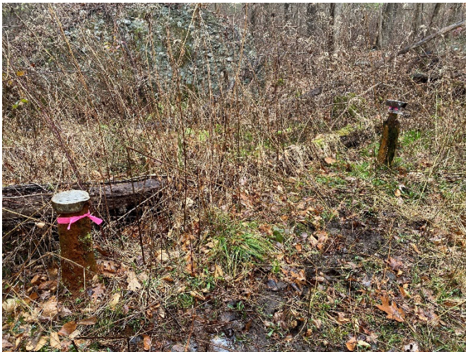
Photograph #27 Groundwater wells MW-7S and 7D (remaining casing shown). Remaining protective casing continuing to rust due to high groundwater and surcharged conditions in standpipe.
